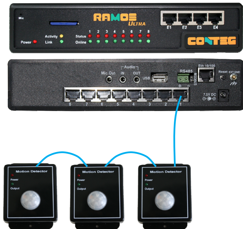
This demonstrates the connection of 3 motion detectors.
